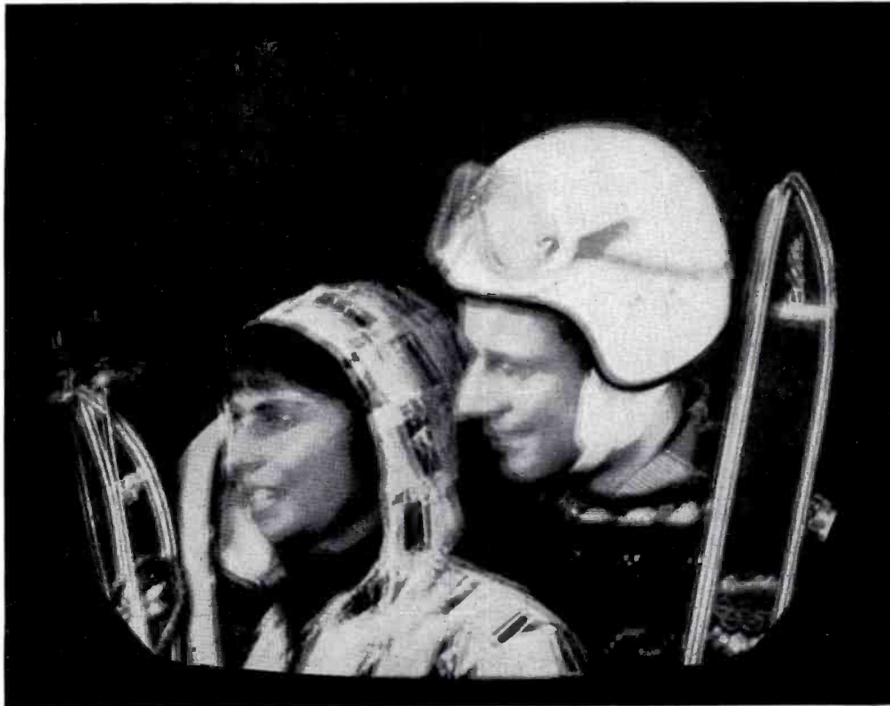
FIG. 3A. Monochrome Picture from Misregistered RGB Camera.
