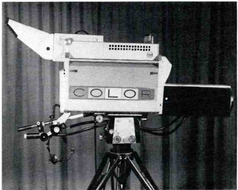
FIG. 5. Focus controls are grouped for easy operation by one hand. Viewfinder and zoom lens assembly are detachable from camera head for easy portability.
