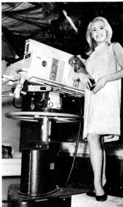
Donna Rae Wood smiles engagingly as she cradles No. 4536 like the newborn 4½-inch image orthicon that it is. New pickup tube that reduces signal-to-noise ratio made its debut in TK-42/43 cameras.
