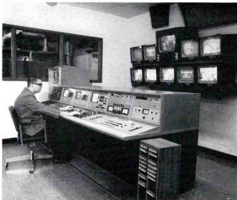
FIG. 3. Operator Dick Clay at the console in master control handles the station breaks while at the same time is able to watch the operation of the transmitter.
