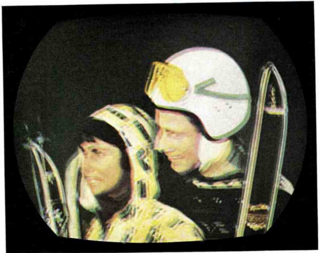
FIG. 3C. Color Picture from Misregistered RGB Camera.
