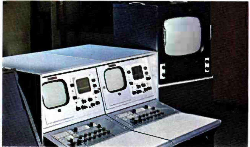
FIG. 2. Two TK-42 Camera controls installed at KHQ-TV. Auxiliary equipment is mounted in these cabinets.
