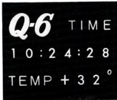
FIG. 10. Time and temperature are displayed by computer type readouts, picked up by a vidicon camera and fed to two color encoders for producing a two-color picture.
